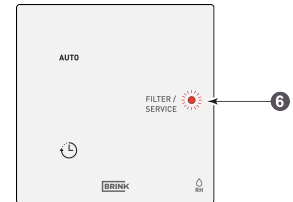
6 = LED fault indication (flashes 1Hz)
