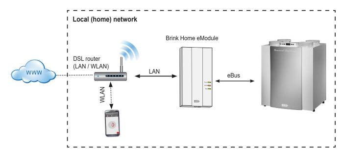
Using the router WPS function (WiFi Protected Setup), it only takes the push of a button to connect the Brink Home Module to the WLAN network. The router does have to support the WPS function (see router manual).
