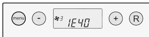
Blokkerende storing; ventilator storing
